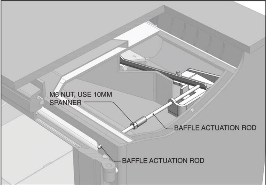
The bypass baffle can be adjusted by undoing the M6 nut and rotating the baffle actuation rod in or out, then retighten the M6 nut. Close the door and check the position of the bypass baffle, it should fit flush to the main baffle when the stove is cold. The bypass baffle will not fit flush with the main baffle when the stove is under fire.
