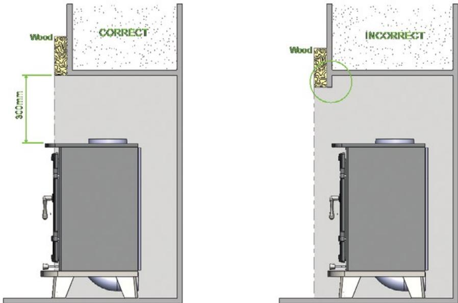
The closure plate must be fitted in such a way it does not allow the build up heat in the fire chamber i.e. flush as shown, the stove must also be in line or protruding forward beyond the fire chamber. The regulations governing connecting flue pipes must be adhered to.
