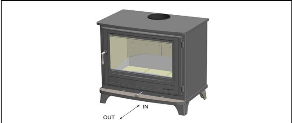
With the air control bar fully out the maximum air is entering the stove at the top front (air wash) and through the rear bricks. When the air control bar is pushed in the air is reduced proportionally between the air wash and the rear brick to give the best "burn". When the air control bar is fully in there is still air entering the stove via the air wash. Before lighting the stove ensure the baffle by-pass is free to operate.
