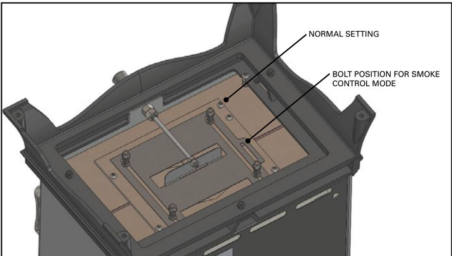
**5WS, 8WS 6kW, 8WS 8kW and 12 Wood Burning Stove Smoke Control:**
