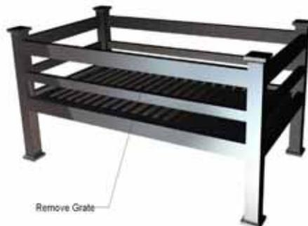
On certain types of fire baskets (mainly curved baskets) both grate structure bars must be removed to enable the fitting of the burner unit.
