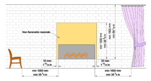
How to construct the housing for the appliance:
