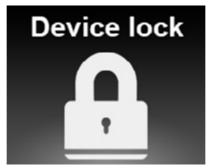
The device cannot be turned on either via remote control, configured device or according to the manual, without previously unlocking it. To unlock the device hold **START/STOP** button for 5s – the message will disappear.
