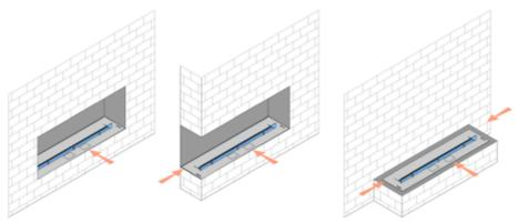
Situations in which installation of a glass shield is forbidden:
