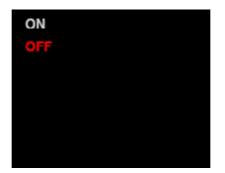
Using "+" button choose OFF option and confirm with "-" button. The device automatically returns to main display and 'Fast start' function will be turned off.
