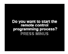
Press "-" button to confirm. Then press in sequence (hold until next message appears) **START**, **STOP**, **PLUS**, **MINUS**. After the remote control has been programmed the messages disappear and main display appears. Remote control is programmed.
