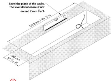
Highlighted  $\bigcirc$  button indicates proper connection of the appliance to the power supply. Once connected to the power source the appliance should be placed in the prepared cavity, by using attached handles. Please make sure to remove the handles before starting the appliance and keep them for the lifetime of the appliance. If necessary, use the handles to remove the appliance.
