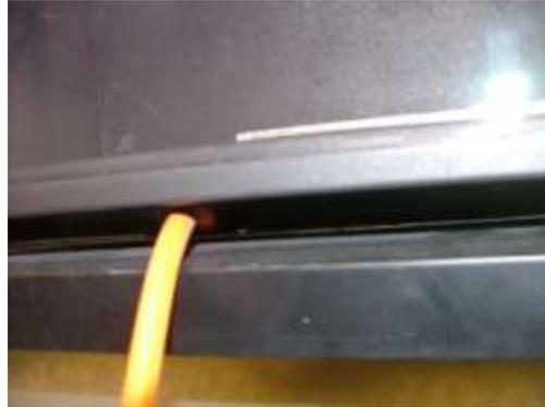
Ensure the wiring is away from the burner base and making sure no wiring is trapped in-between any metal work.
