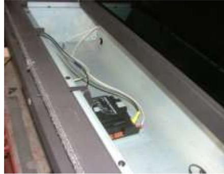
Carefully pull the base back plate out, the TTB bullet connections are threaded through the plate hole (see fig. 41-44).
