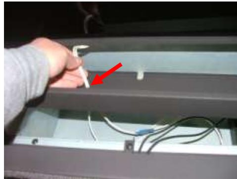
Undo the 4 screws at the back of the appliance to release the TTB (see fig. 76). Attach the two white right angled female connections to the TTB (see Fig. 77). Refit the access panel (Fig. 76).
