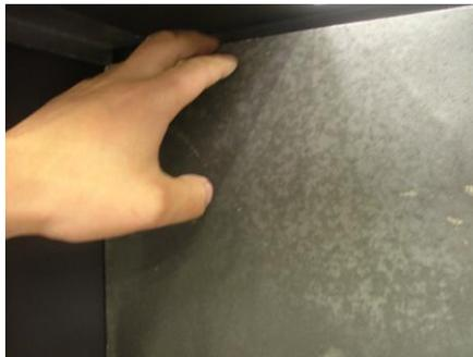
Carefully lift the back panel out (see fig. 129) over the burner. The burner assembly may have to be removed when fitting or removing thicker panels.
