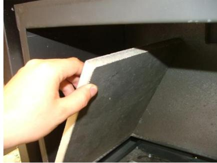
Remove the panel bracket and screw on the opposite side (mirror image of fig. 126), lift the side panel out (see fig. 127) hold back the back panel at the same time to ensure it doesn't fall. (see fig. 128)
