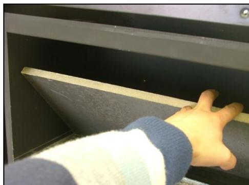
Fit the side panels securing in place using the adjustable brackets and screws (see fig. 55).
