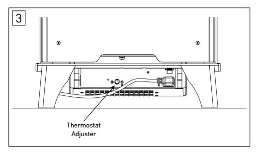
just click off. The heater will then maintain the room temperature at the chosen level. Apart from innitial fine tuning the thermostat is designed and positioned not for continual resetting (fig3).
