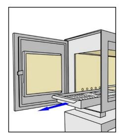
add a couple of firelighters. You then simply push the trays part-way back into position and light the firelighters. Once the firelighters have caught, you should then carefully push the trays back all the way back in and position the doors, so they remain slightly ajar, to aid airflow. Once the kindling is fully alight, you can close the doors, though if the fire dies back, keep them open until you can close without any change in the fire.
