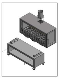
The flue collar is secured to the top of the unit with the 4 screws provided. Once secured in place, you can slide over the 6" flue section, rain cap and finishing angled ring to meet with the top of the fire box.
