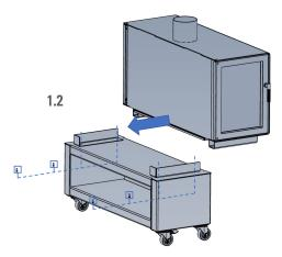
Take care not to trap hand/finger between the two units. Once in position secure the main burner unit to the log store base using the 4x bolts and washers provided (Diagram 1.2). If you wish to move the unit at any point ensure that the two units are fixed together properly.
