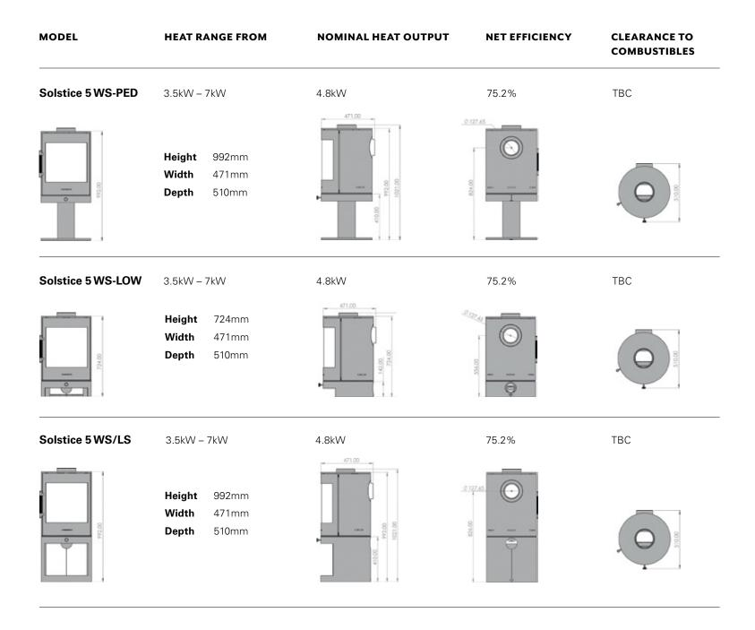
FLUE OUTLET Solstice models Top Flue outlet 150mm : Rear Flue outlet 125mm
