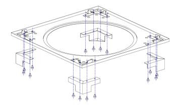
Place 1x long panel and 1 x short panel at 90 degrees to one another in the locating bracket on the base plate. Secure the panels in place by fitting the top angle bracket\*. Tighten the fasteners top and bottom until secure. Do not overtighten.
