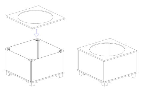
6. Place the fire pit burner through the hole in the countertop in the location grove in the centre of the base plate
