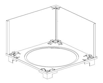
\* When using teak panels replace the screws in the top angle brackets with the shorter screws provided.
