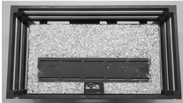
Typical burner in basket showing black insulation pad in position and vermiculite fill, ready to lay ceramics
