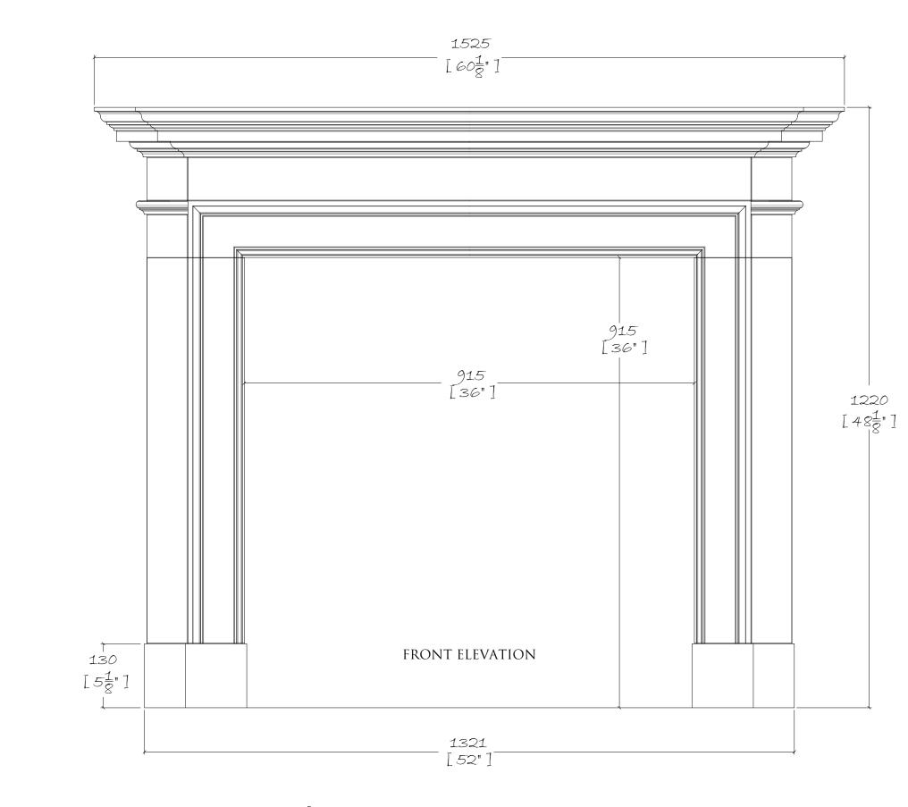
SHELF DEPTH - 224mm - 8 <sup>7</sup>/<sub>8</sub>" Standard Rebate for SLIPS - 25mm - 1"
