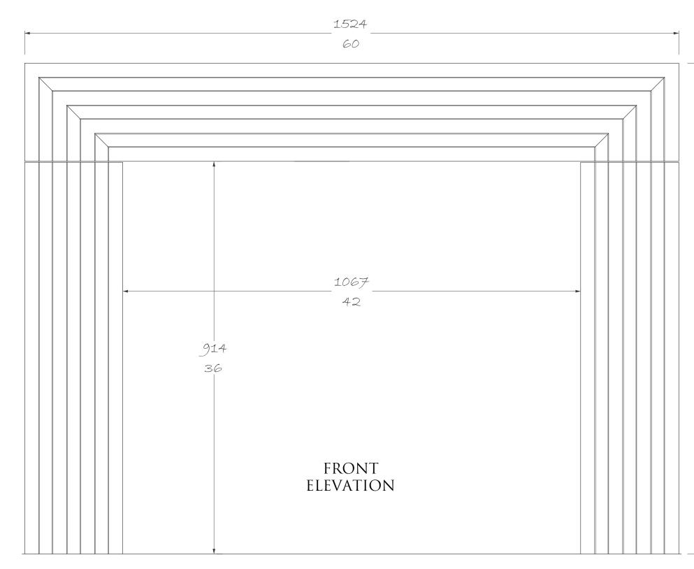
STANDARD REBATE FOR SLIPS - 25mm - 1" DEPTH OF JAMB - 171mm - 6 <sup>3</sup>/<sub>4</sub>"
