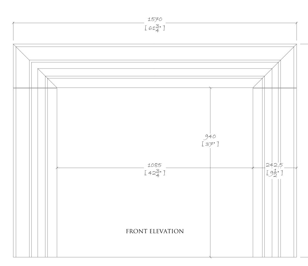
STANDARD REBATE FOR SLIPS - 25mm - 1" DEPTH OF JAMB - 180mm - 7 <sup>1</sup>/<sub>8</sub>"
